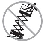
Do not drive the machine on or near uneven terrain. unstable surfaces or other hazardous conditions with the platform raised.
